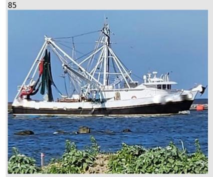
Asking Price: \$395,000. Size: 85' x 20' x 10' Material: Steel Main Engine: KTA19 Cummins Horsepower: 600 Gear Ratio: 6:1 Generators: (2) — 6B Cummins 65kW (Both rebuilt) Fresh water tank capacity: 7,000 gallons
