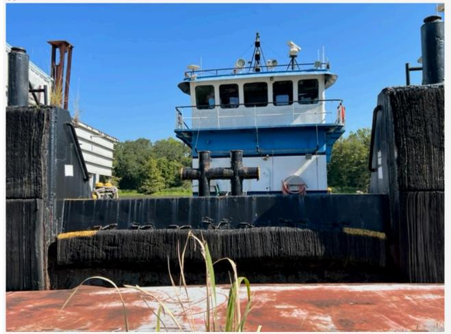
Asking Price: \$530,000. Size: 65' x 24' x 9' Type: Square Bow Lugger Horsepower: 900 Draft: 6'6" Deck Space: 25' x 22' Year Built: 1982 Speed: 10 MPH Main Engines: (2) - John Deere ...
