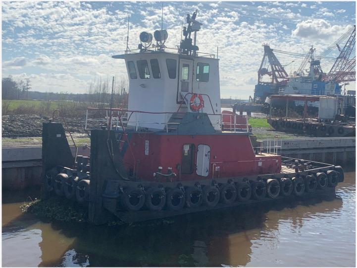
Asking Price: \$450,000. Size: 50' x 20' Type: Pushboat Horsepower: 600 HP Year Built: 1979 Main Engines: (2) - Detroit 8V71 (600 HP) Generators: (2) - Isuzu 4B61 40KW Berths: 3 Fuel: 5,000 USG
